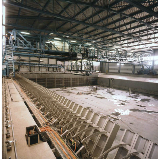
Figure 1.2: The wave-current basin of MARIN without water. The current culverts are visible at the farthest side
