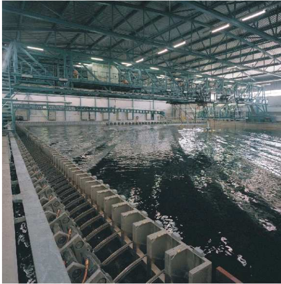
Figure 1.1: The new offshore (wave-current basin) of MARIN. The individually controlled flaps of the wavemaker on the longitudinal side of the basin are clearly visible on the left foreground. The other series of flaps are located at the farthest side. Source: [43]
